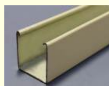
V16-01-1 STEEL HEAD RAIL, 19mm x 22mm, PAINTED 20pcs/ctn, 4meter/pc
